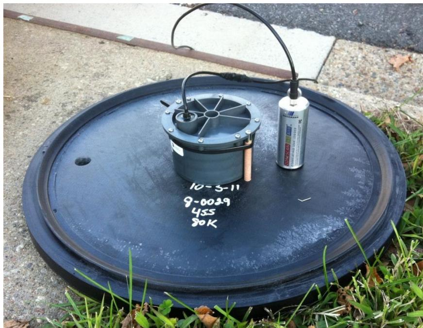
Figure 2.1 Acoustic logger modified to transmit results on a fixed AMI network
