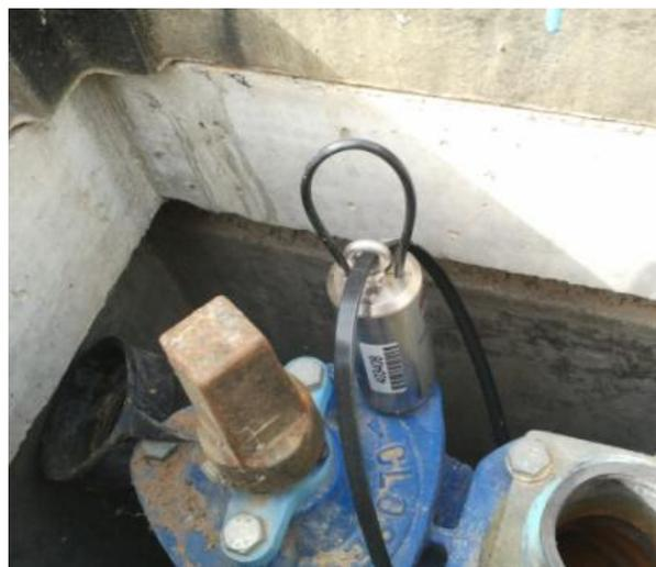
**Figure 1.6 Correlating noise logger secured on hydrant with a steel cable tie.**
