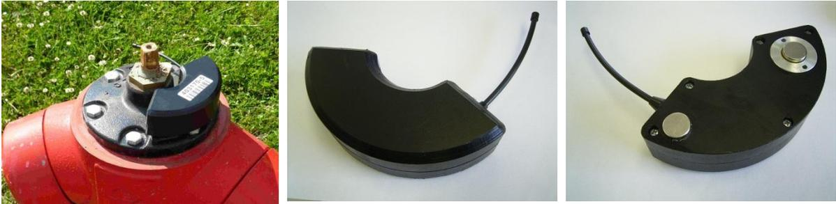
**Figure 1.5 Pictures of an acoustic logger developed to fit onto above ground hydrants**
