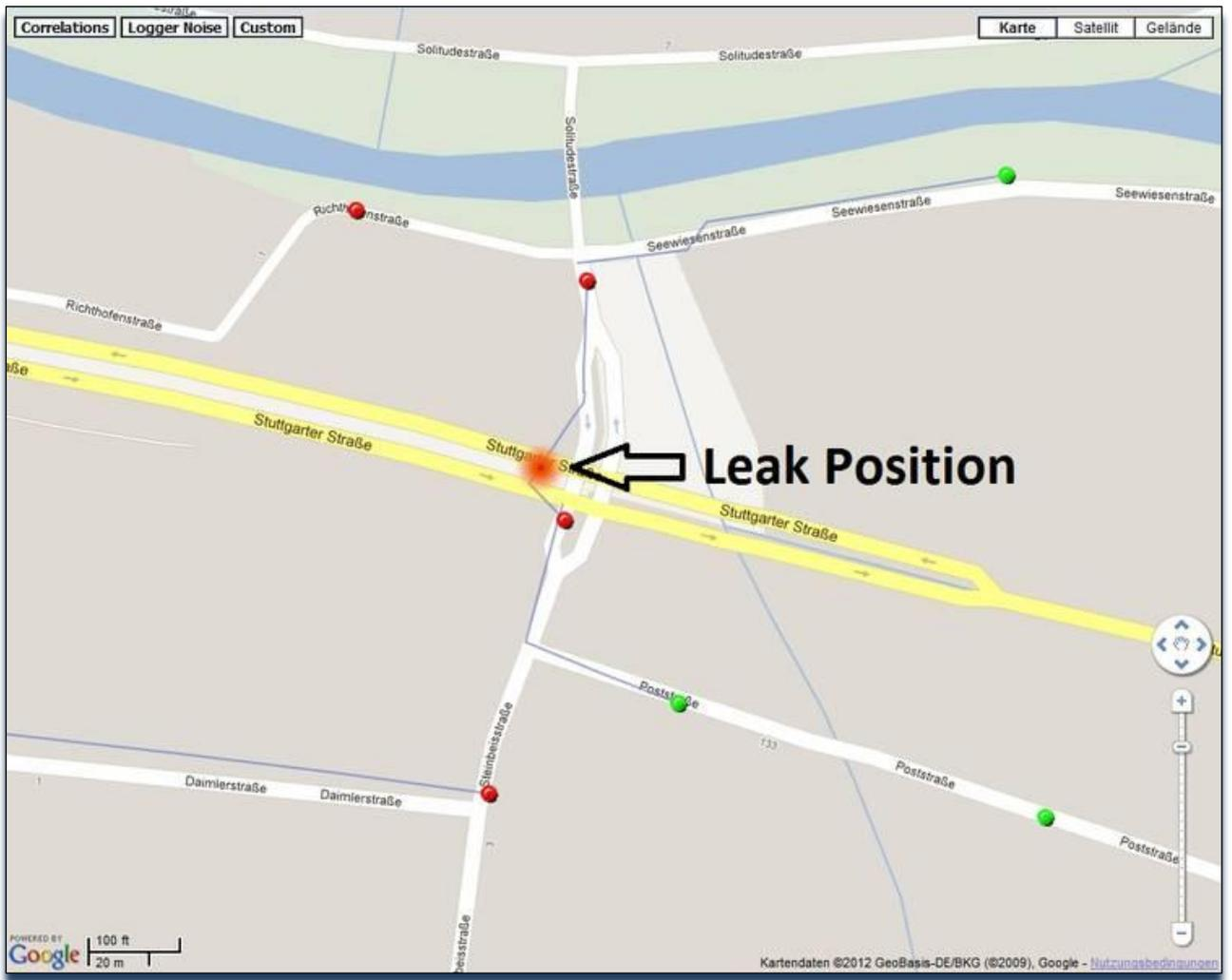
Figure 4 Map from ZoneScan NET software (Red dots = High noise logger positions / Arrow = correlations / Fuzzy orange dot is leak position)
