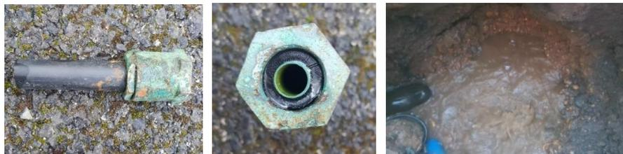
*Figure 5 - Excavation reveals leak on plastic communication pipe*
